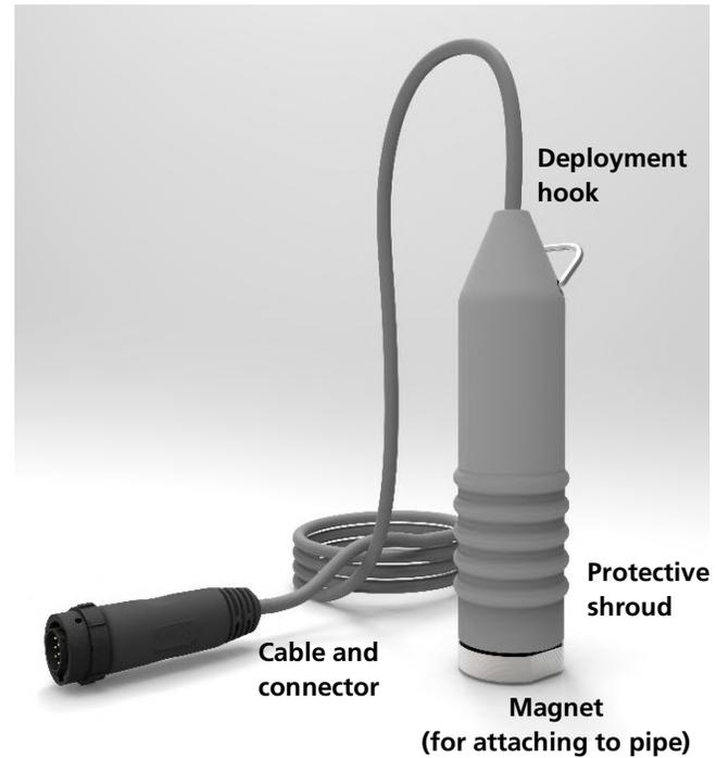
**Option for Plastic Pipes & Large Diameter pipes :** The Touch Pro can also be optionally **utilized with hydrophone sensors** which are utilized in difficult operating conditions where they are mounted for direct contact with water column at hydrant, air valve or flow meter points (pressurised water) - Hydrophones are also more ideally suited for large diameter trunk leaks and all types of plastic pipe systems, and detects the noise signals travelling within the water column itself.
