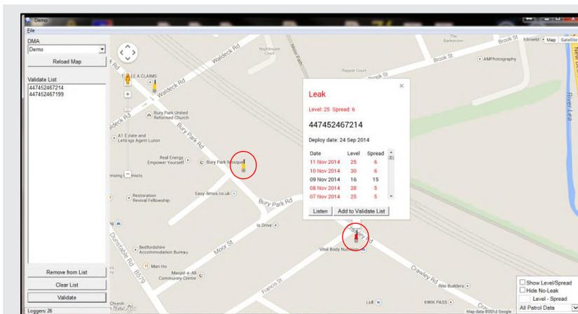
Sites coloured Yellow are not detecting a leak, Red sites are where a leak is suspected.
