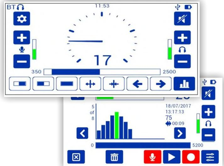
**Water Leak Indication :** When moving along the path of a given water pipe, the closer you get to the leak point, the signals received from the leakage will grow in intensity and/or range. The noise heard becomes louder and larger horizontal signal bar-graphs are displayed on the screen.
