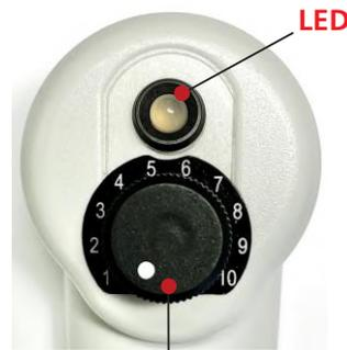
Top view of the Lmic showing the rotary control for volume and sensitivity.
