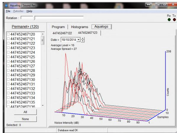
**Histograms & Aqualogs:** Additionally, the leak detection team can view daily Histograms of individual loggers, or via detailed Aqualogs including 3D views.
